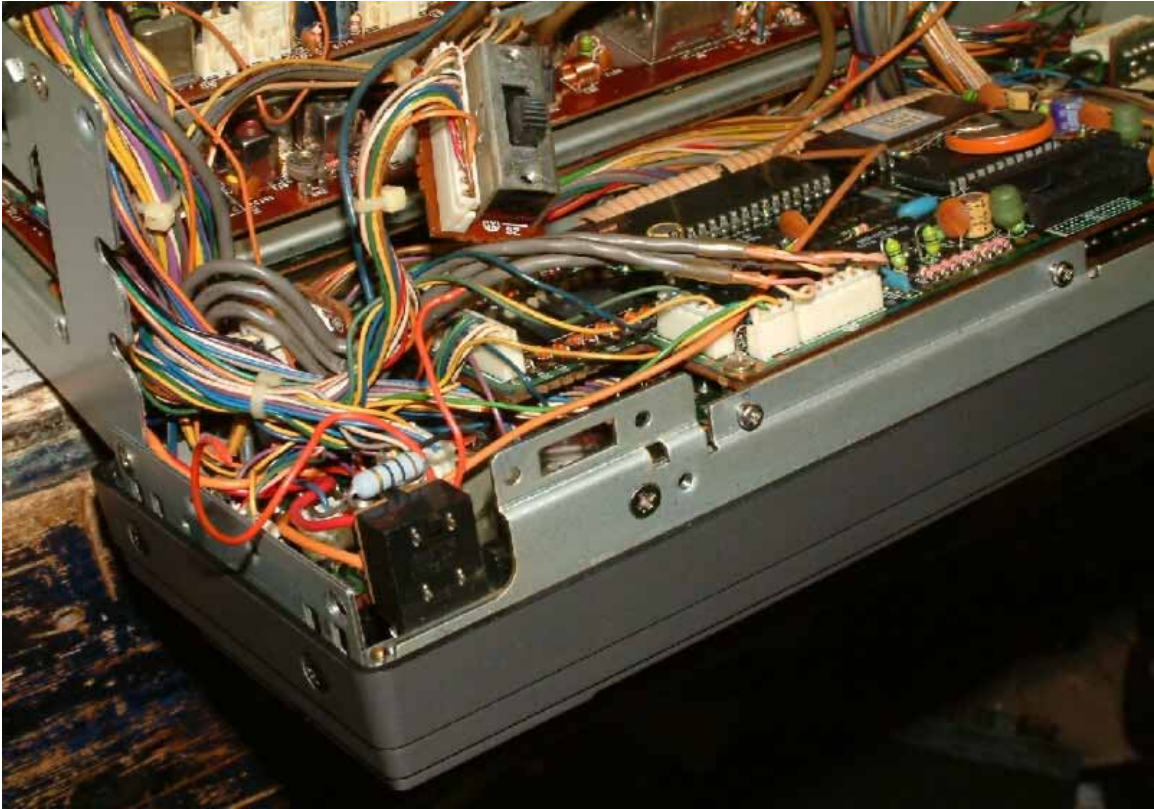
Picture 3: After switch removed (note that the wires are long enough that the switch can be tied back out of the way).
