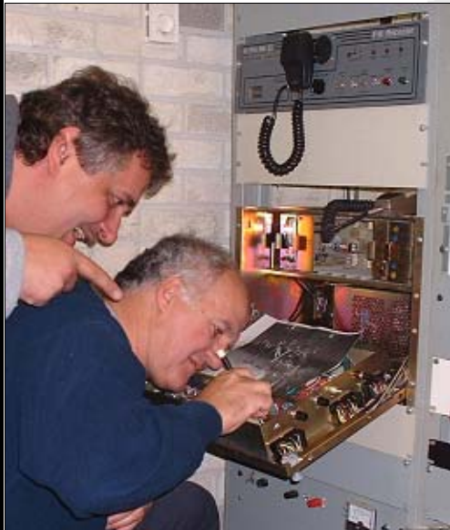
Tedd VE3TJD and Dave VA3MRJ shown adding the Tone Squelch Encoder to the new KSR. The old KSR is at the top right of the photo
