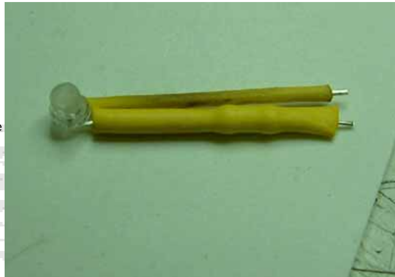
After the resistor is installed, cover both leads with heat shrink tubing and trim the leads to be the same length.
