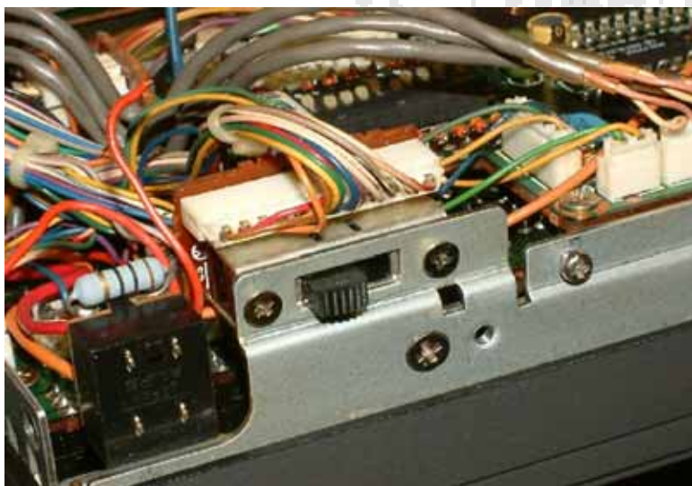
Here is the switch before removal
