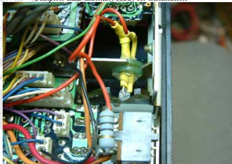
Completed LED assembly in it's new home! Tuck the wires so that they don't get pinched when you put the CW/VOX switch or the display unit back in place.
